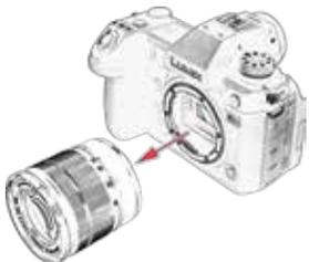
Remove the L-Mount lens from the L-Mount Alliance interchangeable lens camera by depressing the lens release on the front of the camera, turning counterclockwise until the orientation marks are aligned, then pull the lens away from the camera body. Keep the rear optic of your L-Mount lens protected with a rear lens cap.
