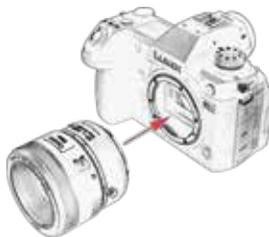
While the L-Mount Alliance camera is turned off, install the lens / adapter assembly by lining up the orientation marks on the rear of the adapter and front of the camera, inserting the adapter into the camera's lens mount then turning clockwise until you here a click which indicates the assembly is safely locked into place on the camera.
