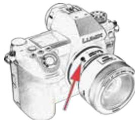
The 'Fn' button disables all electronic communication between the lens and camera. Ideal for shooting video where you want full control over the focus of the lens or if you want to use the lens/camera combination in full manual mode.
